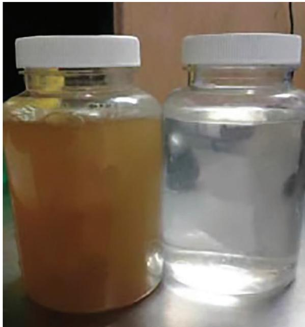
*Before and after treatment of produced water for fracturing reuse with the RenewIQ solution.*
