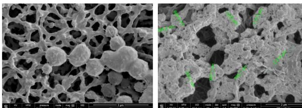
**Figure 2.** Scanning electron microscopy (SEM) images of cellulose nitrate filter; unused filter (left) and filter after filtration of liquid cracker PW (right).
